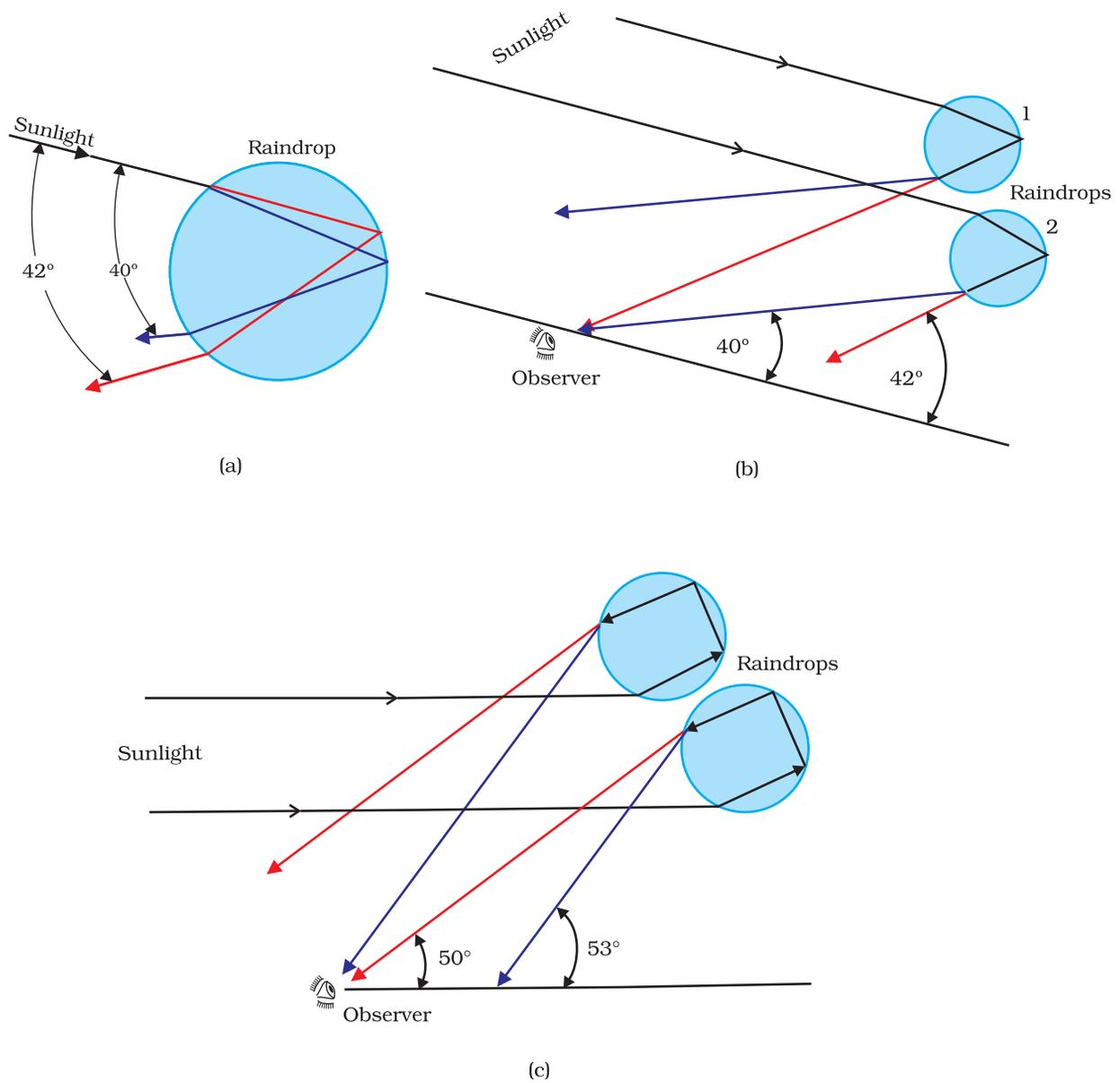
**FIGURE 9.27** Rainbow: (a) The sun rays incident on a water drop get refracted twice and reflected internally by a drop; (b) Enlarge view of internal reflection and refraction of a ray of light inside a drop from primary rainbow; and (c) secondary rainbow is formed by rays undergoing internal reflection twice inside the drop.
