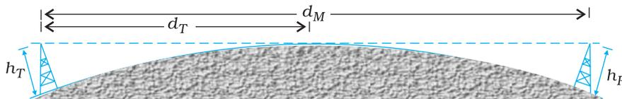
**FIGURE 15.5** Line of sight communication by space waves.
