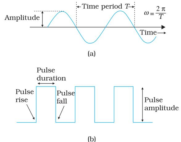
**FIGURE 15.7** (a) Sinusoidal, and (b) pulse shaped signals.
