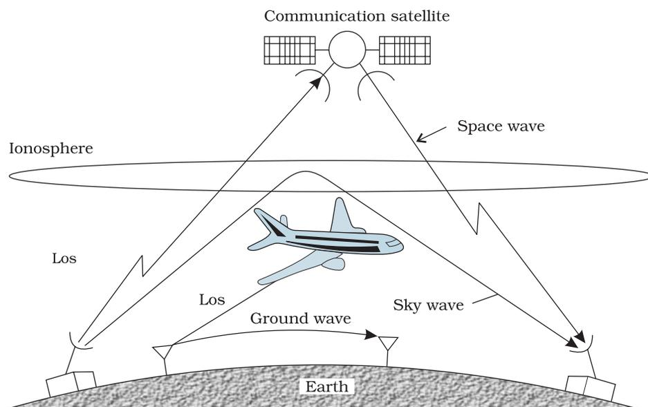
FIGURE 15.6 Various propagation modes for em waves.
