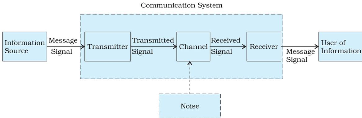
**FIGURE 15.1** Block diagram of a generalised communication system.
