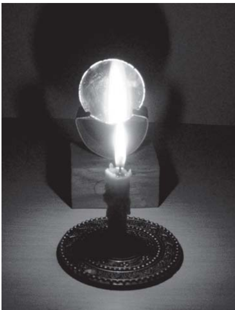
Fig. 15.16 Virtual image formed by a concave mirror
